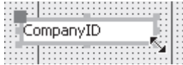
Figure 11-13 You can drag a corner handle of a selected control to change the control's width or height or both.
