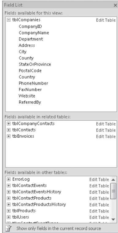
Figure 11-7 The field list shows the names of the fields in the bound table or query, any related tables, and fields from all other tables in the current database.
