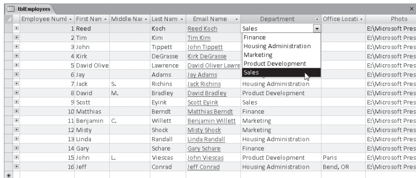
Figure 5-35 The Lookup tab settings show you a combo box in Datasheet view.
