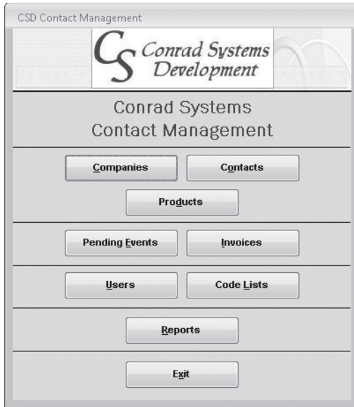
Figure 10-21 The command buttons on the frmMain switchboard form take the user to various parts of the application.
