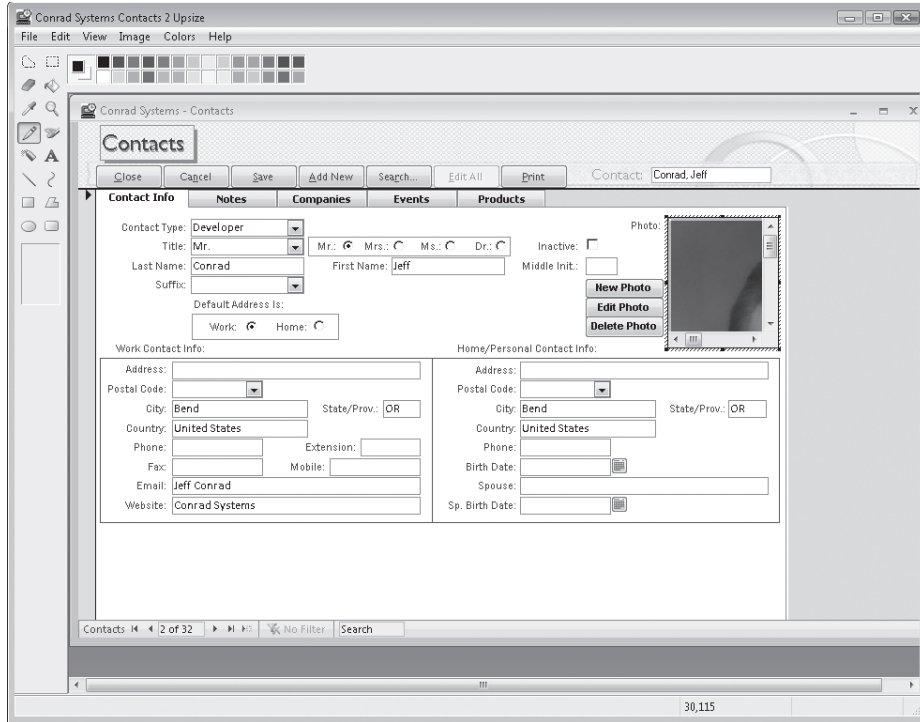
Figure 10-20 The Photo OLE object field from Figure 10-19 is being edited “in place” with its host application.
