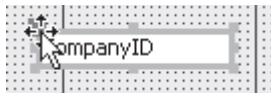
Figure 11-15 You can drag the large handle of a selected control to move the control independently of its label.
